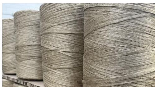
Fig. 1 Flax fiber roving [Depestele]
